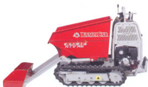
CASSONE DUMPER CON AUTORICARICANTE DUMPER TYPE BODY COMPLETE WITH SELF-LOADING FRONT BUCKET R 70 - R 70 PLUS
